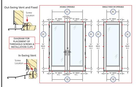
C. Doors using Installation Clips: Install installation clips. Place each clip so the lip is facing up and against the installation fin at the locations shown in the placement diagram. Secure each clip by driving a  $#6 \times 5/8$ " corrosion resistant screw through each of the outer two holes of the three holes shown.
